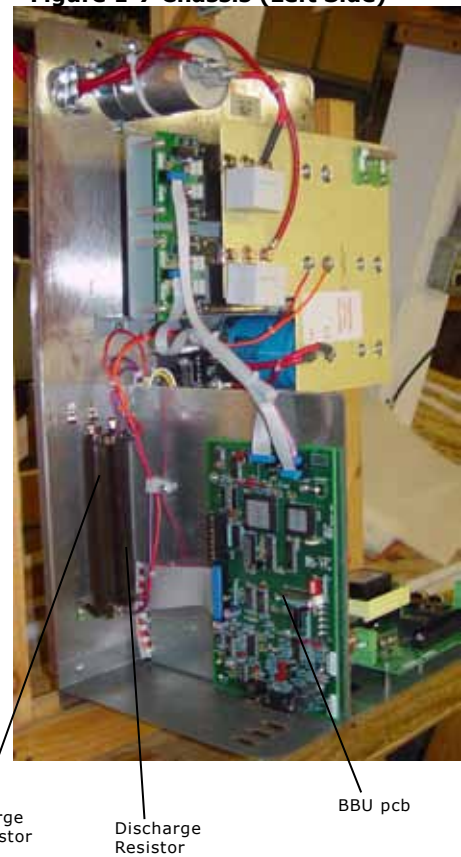
Figure 1-7 Chassis (Left Side)
